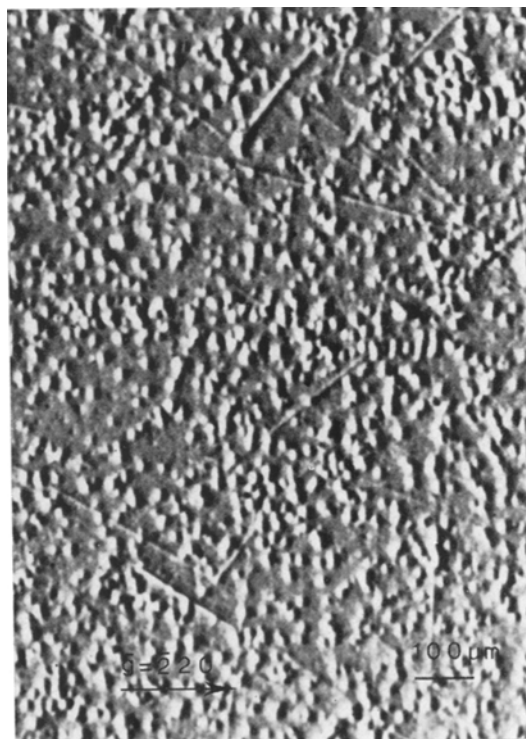
Figure 1 \bar{2}20 X-ray topograph showing precipitates in P-diffused (111) silicon. \text{CuK}\alpha_1 radiation.
